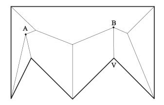
Figure 3: Reflex vertex can yield to both cases: an edge event (point A) or a split event (point B)
